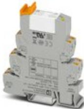
PLC-INTERFACE, consisting of PLC-BPT.../21-21 basic terminal block with Push-in connection and plug-in miniature relay with multi-layer gold contact, for mounting on DIN rail NS 35/7,5, 2 changeover contacts, input voltage 24 V AC/DC
