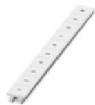
Zack marker strip, Strip, white, labeled, can be labeled with: CMS-P1-PLOTTER, printed horizontally: consecutive numbers 1 ... 10, 11 ... 20, etc. up to 91 ... 100, mounting type: snap into tall marker groove, for terminal block width: 10.2 mm, lettering field size: 10.15 x 10.5 mm, Number of individual labels: 10
