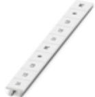
Marker for terminal blocks, Strip, white, labeled, can be labeled with: CMS-P1-PLOTTER, horizontal: L1, L2, L3, N, PE, L1, L2, L3, N, PE, mounting type: snap into tall marker groove, for terminal block width: 10.2 mm, lettering field size: 10.15 x 10.5 mm, Number of individual labels: 10
